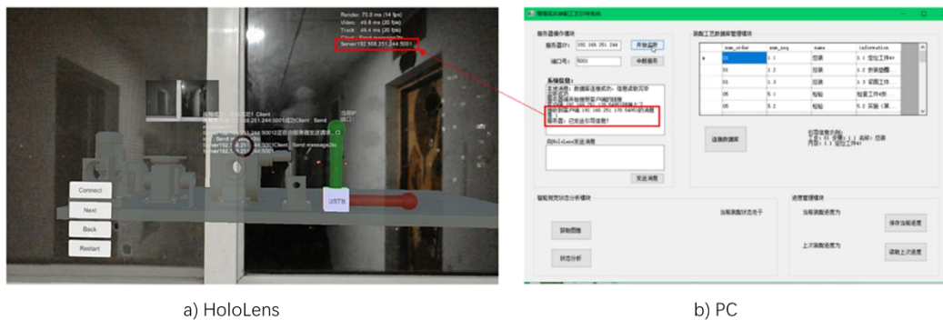
Figure 10. Asynchronous socket communication between PC and HoloLens.
