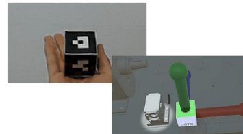
Figure 7. 3D registration and virtual-real integration.
